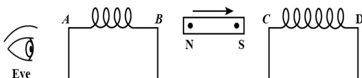
A bar magnet NS is moved in the direction indicated by an arrow between two coils AB and CD as shown in the figure. in which Coil the direction of current will look like anti- clockwise if viewed from left side ?
