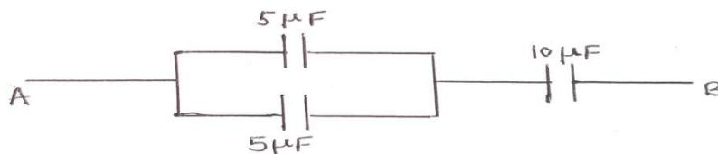
Calculate the equivalent capacity of the combination of capacitors between A and B in given diagram.
