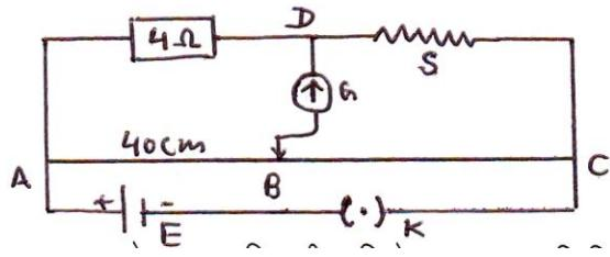
In the given circuit diagram, find the value of unknown resistance  $S$ , in the balancing condition of meter bridge.
